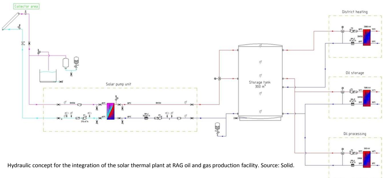
Hydraulic concept for the integration of the solar thermal plant at RAG oil and gas production facility. Source: Solid.
