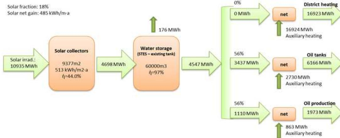
Simulation results for the variant with a reconversion of one of the oil tanks into a STES. Solar system heat balance including a STES with 60.000 m<sup>3</sup> (one of the existing tanks) and reduced set point temperatures for the collector circuit. Datasource: Solites, Graphics: Tecnalía
