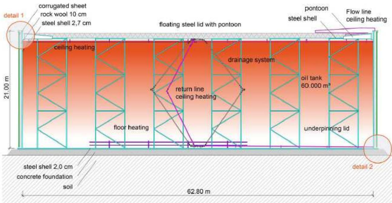
Reconversion solution for the existing tank of 60,000 m<sup>3</sup> to be used as STES. Source: Solites.
