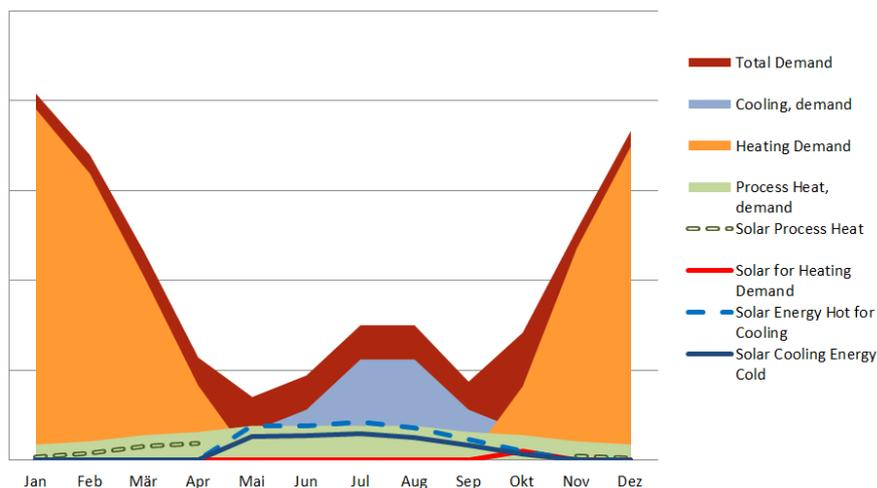
**Figure 4: Heating and cooling demand and supply over the year of the project at AVL List GmbH.**
