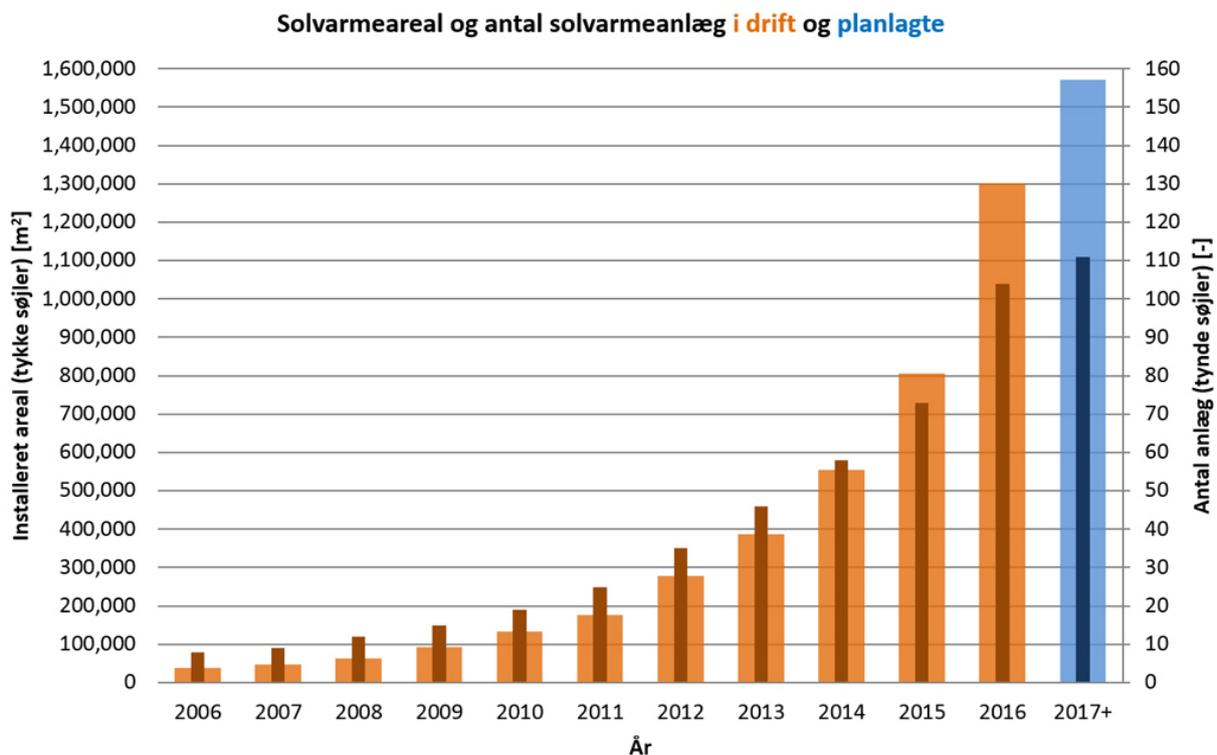
**Figure 5. Development of solar thermal installations in terms of installed collector field area (left) and numbers of systems (right), orange are the already installed systems and blue the planned installation for 2017; (Source: Per Alex Sørensen, PlanEnergi)**
